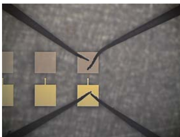
20x20 \mu\text{m} C = 857 \text{ fF}
