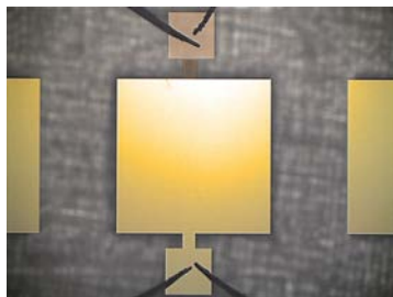
1000x1000 \mu\text{m} C = 1.6 \text{ nF}
